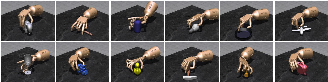
Fig. 6: Examples of pre-grasps used in our experiments. Note how they (1) place the hand in proximity to the target object and (2) and pose the fingers around functional parts of the object (e.g. hammer’s handle). However, pre-grasps are not stable grasps. In fact, the hand does not make contact with the objects at all!
